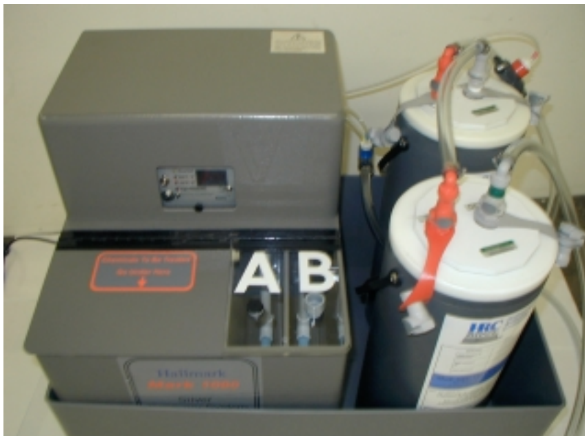
Illustration 2: Orientation and Hookup of the Filter Columns
